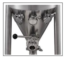
• Assemble the elbow pipe to the 2" TC port at bottom with clamp. Do not forget to place the gasket at the groove in between. Then attach the 2" TC butterfly valve to the elbow with the gasket in between and clamp tighten it on.
